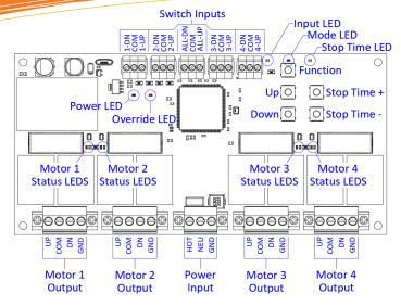
IMPORTANT: If both left and right hand motor configurations are used, UP and DOWN wires for individual motor outputs may need to be swapped in order to function correctly with grouped switches. To verify wiring, all motors should run in the same direction when operated from the onboard UP/DOWN buttons.
