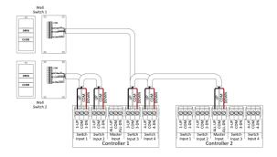
Motors 3 and 4 on Controller 1 and all motors on Controller 2 operate from Wall Switch 1
